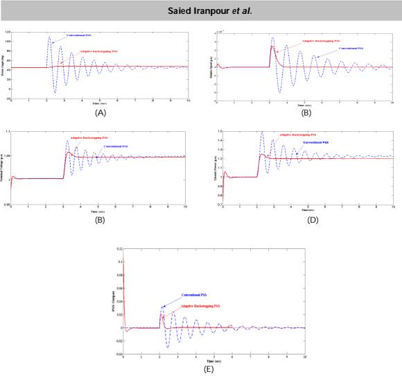
Figure 5: For 20% of change in mechanical power: (A) rotor angle change; (B) Changes in velocity; (C) variations of electrical power; (D) changes in terminal voltage; (E) PSS output.
