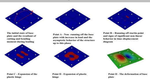
Figure 10 - The process of destruction of base plate connection - sample 1 - (zoom ratio: 2)
