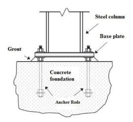
Figure 1 - A view from the the constituents of the column bottom connections in steel structures
