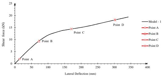
Figure 8 - Diagram of load-horizontal shift for models 1
