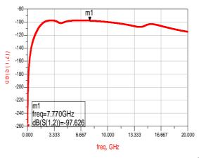
Fig. 14. The factor associated with inverse isolation (S12)
