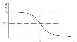
Fig. 4. The frequency response of low-pass Butterworth
