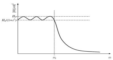
fig. 5. Frequency response of the Chebichov filter
