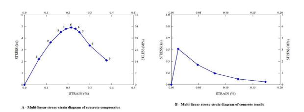
Figure 4 concrete compressive and tensile stress-strain curve - derived from experimental Opening size of 5 mm Due to lack of continuity of the weld
