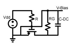
Fig. 8. Biasing circuit of transistor
