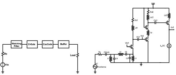
Fig. 1. The structure of proposed amplifier
