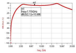
Fig. 13. The factor associated with power gain (S21 (db))
