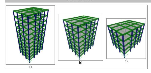
Figure 2: a) 5-story structure, b) 8-story structure, c) 12-story structure
