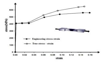
Figure 3 The stress-strain diagram for steel
