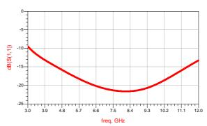
Fig. 11. The factor associated with input impedance matching (S11 (db)),
