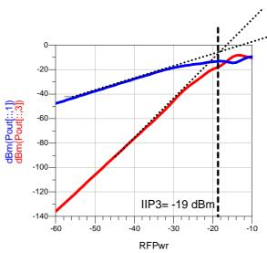
Fig. 15. IIP3 calculation with crossing method (IIP3= -19 dBm)
