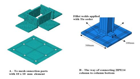
Figure 5: A view of meshing and connecting the components of column bottom
