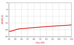
Fig. 12. The factor associated with output impedance matching (S22)
