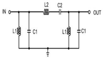
Fig. 6. Band pass filter
