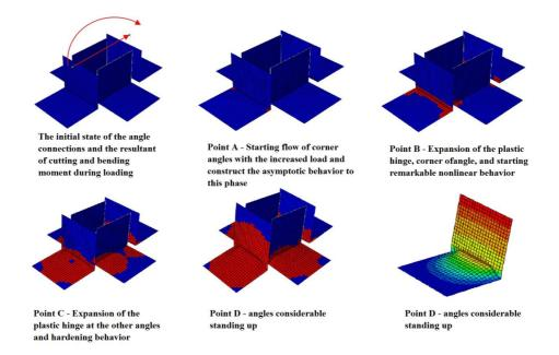
Figure 9 - The process of destruction of column bottom's connection - sample 1 - (zoom ratio: 2)
