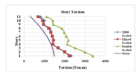
Figure 8: comparison of torsion by different methods
