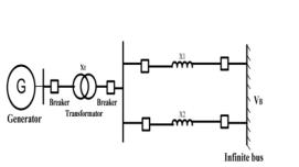
Figure 1: A single machine connected to infinite bus
